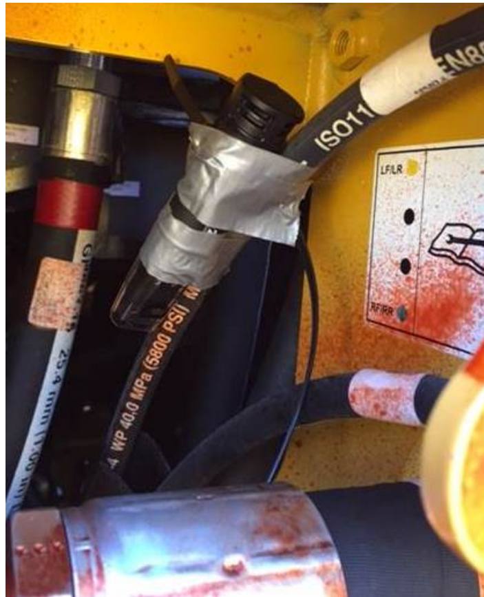
Figure 6: Temperature and humidity sensor attached to hose on vehicle exterior.
