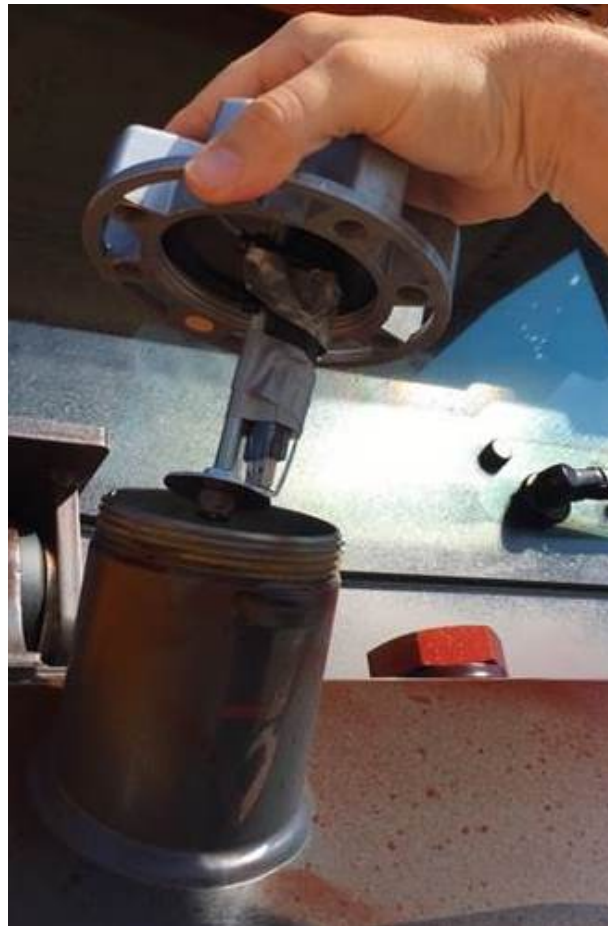
Figure 5: Temperature and humidity sensor attached to modified fuel cap.
