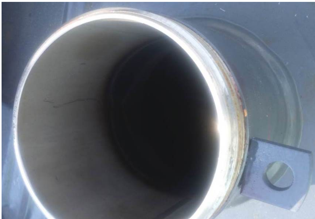
Figure 16: VCI treated fuel tank, after shipment. No corrosion was visible.
