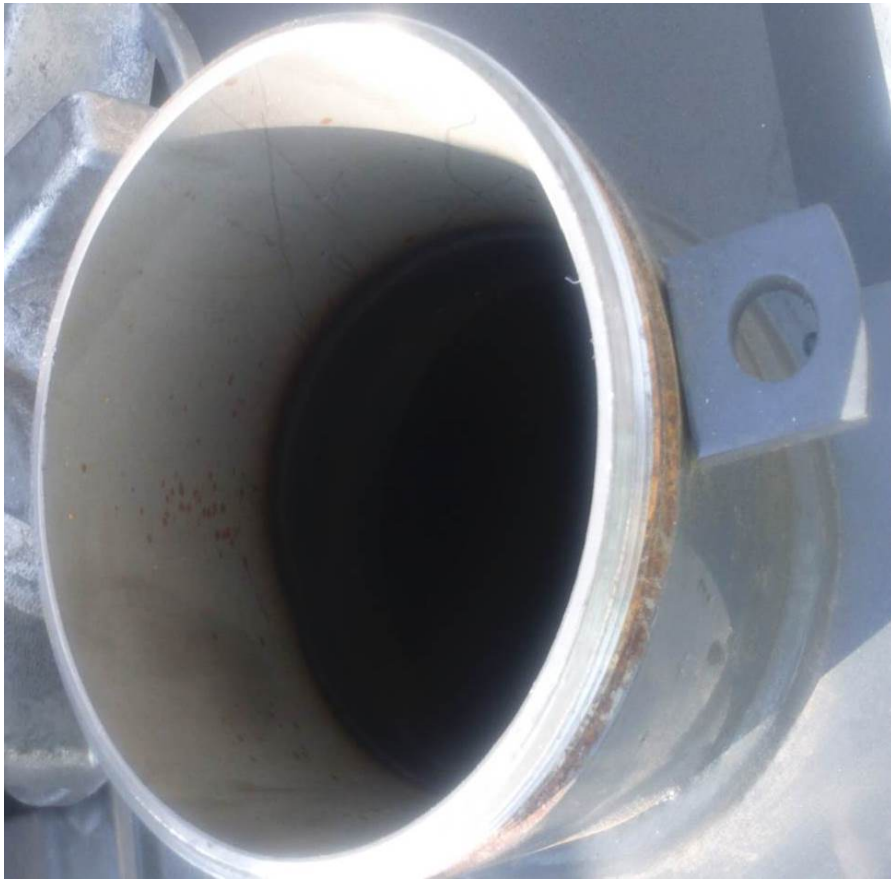
Figure 15: Untreated fuel tank, after shipment. Corrosion is present in the fill neck, which is commonly seen upon receipt inspection.
